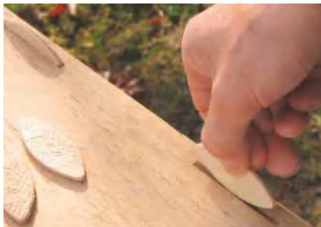
STEP 13. Use No.20 biscuits for fixing the upper shelf to the rear panel. This size is also used for the end pieces
